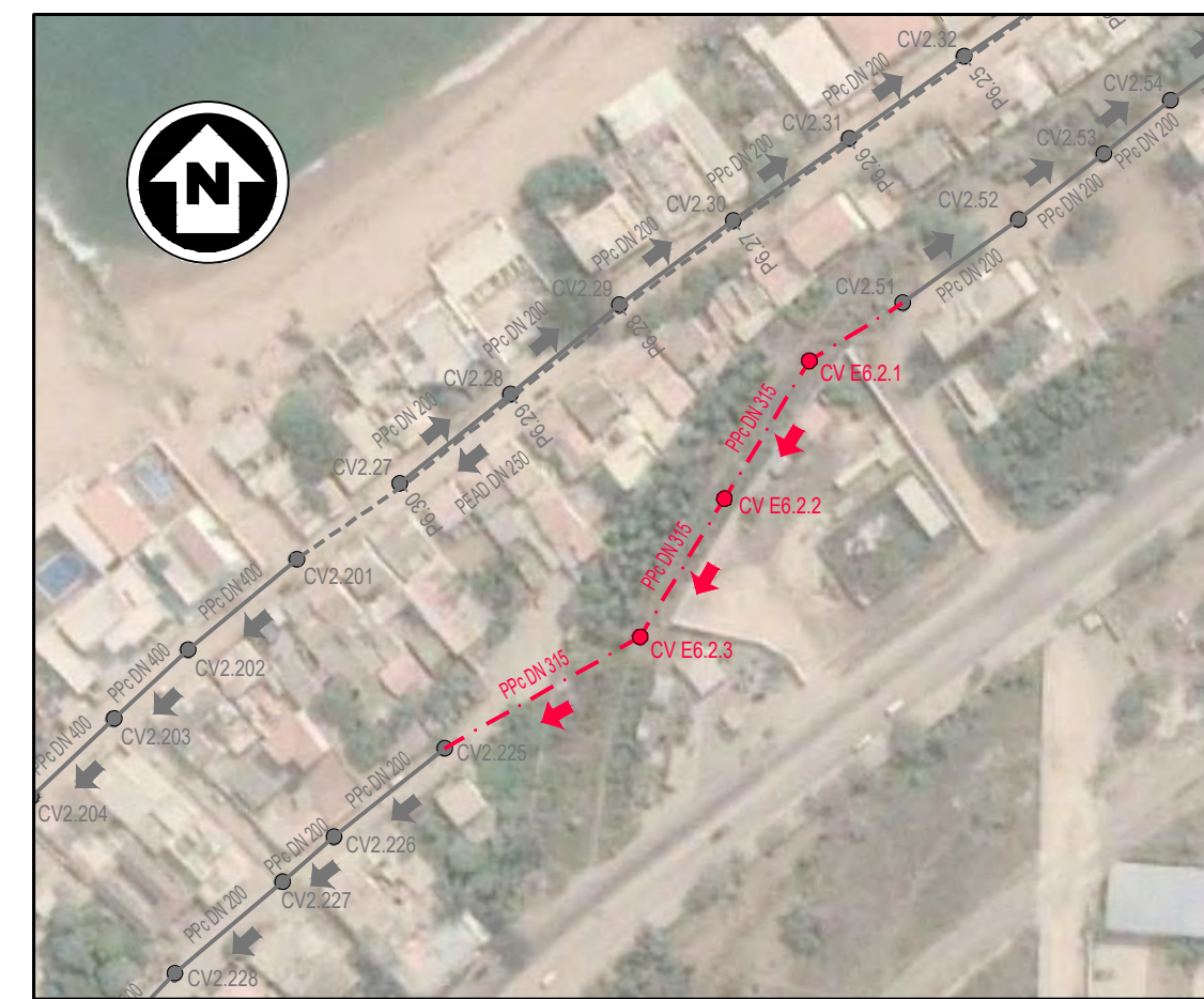
By-pass entre as Bacias 6 e 8 / By-pass Between Catchments 6 and 8 (Escala / Scale - 1/2000)
